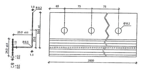
Vertical connection profile – "Verbindungsleiste Alu" (dimensions in millimetres)
